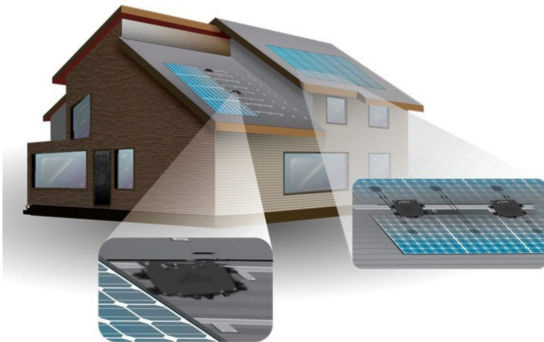
Figure 1: Typical roof-top micro inverter home installation.
