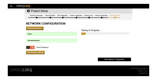
The SparqLinq will take down its Wi-Fi access point and attempt to connect to the wireless network selected using the credentials provided. After testing, it will re-enable its Wi-Fi access point. The installer may need to re-connect to the SparqLinq access point unless "Connect Automatically" was set on the installer's device.
